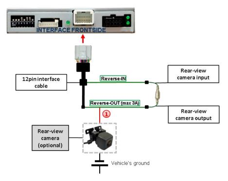
1 Additionally, the +12V (max. 3A) power supply for the rear-view camera can be taken from the green wire of the 12pin interface cable.
