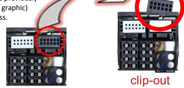
If, after connecting the PNP harness, no interface LED lightens up while the ignition is turned on, the single red wire ACC-out (max 3A) and the purple coloured wire Manual ACC of the 12pin interface cable both have to be connected additionately to S-contact terminal 86s +12V (e.g. glove compartment illumination).
